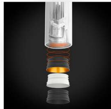
2 optics including reflector and lens and 4 beam angles. Honeycomb filter work as optional. Anti-glare rings is optional in white, black and golden.
