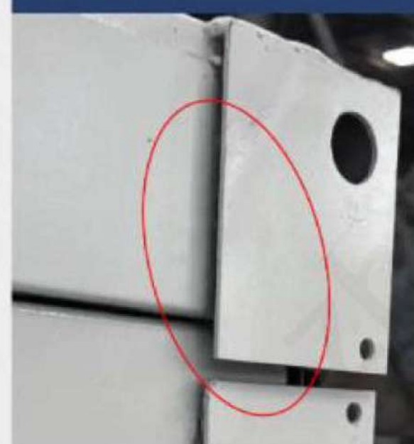
Corner pieces are 2-3mm thick
