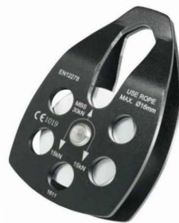
Large single pulley with swivel sides Material: Aluminium Max rope diameter: 16mm ■ EN 12278
