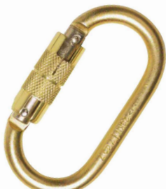
Auto lock oval carabiner Material: Steel Opening: 20mm ▪ EN 362 class B
