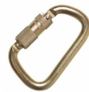
Screw lock oval carabiner Material: Steel Opening: 18mm ▪ EN 362 class B
