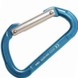
Light carabiner Material: Aluminium Opening: 23mm ▪ EN 12275
