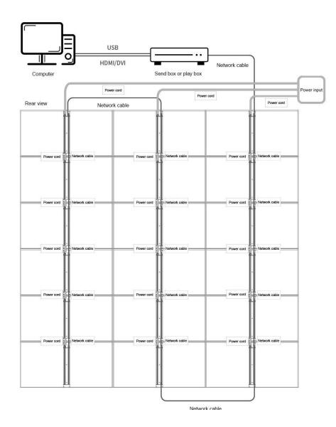
Installation diagram and wiring diagram (synchronous and asynchronous configuration)
