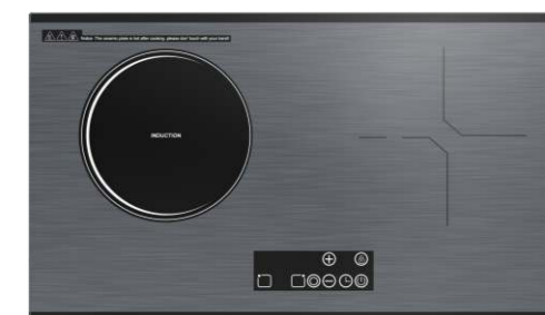
GPS-59 Touch type Power: 2400W+2400W Voltage: 220V/50Hz Panel size: 735*415mm Heating Area: 220mm Iron spray anticorrosive bottom shell/or galvanized sheet
