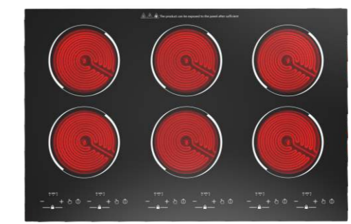
GPS-94 Touch type Power: 1800W+1800W+1800+1800W+1800W+1800W Panel size: 780*510mm Voltage: 220V/50Hz Iron spray anticorrosive bottom shell/or galvanized sheet
