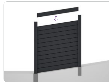
3. Install Fencing Board
