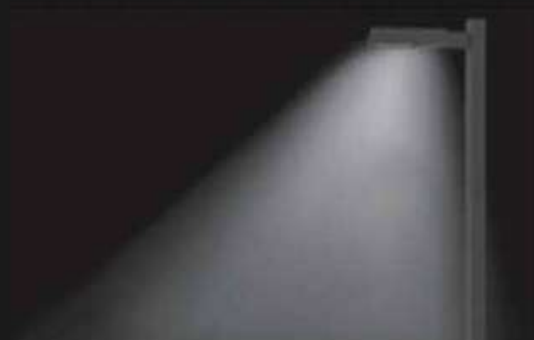
Few light spill behind the pole
