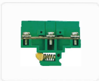
GPS-354 导线截面 wire section: 0.75-2.5mm 2 额定电流/电压 rated current/voltage: 24A/500V 厚/宽/高 thick/wide/high: 54/47/10mm
