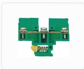
GPS-355 导线截面 wire section: 0.75-2.5mm 2 额定电流/电压 rated current/voltage: 24A/500V 厚/宽/高 thick/wide/high: 54/65/10mm
