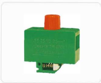
GPS-353 导线截面 wire section: 0.5-2.5mm 2 额定电流/电压 rated current/voltage: 24A/660V 厚/宽/高 thick/wide/high: 12.5/41/48.5mm
