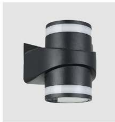
GPS-199 Dimension: 145x140x120mm Lamp: LED 2x5W / 2x7W Voltage: 85-265V Material: Aluminum+Glass+PC
