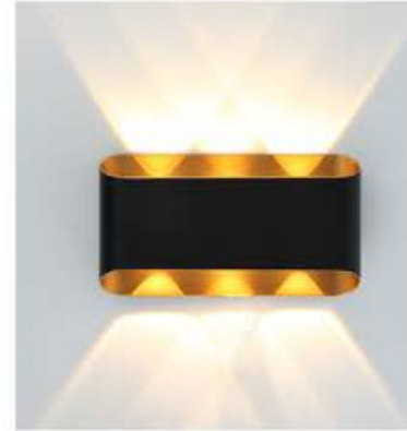
GPS-157 Dimension: 180x35x100mm Lamp: LED 6x1W Voltage: 85-265V Material: Aluminum+PC
