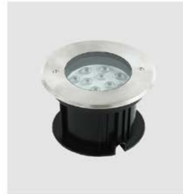
GPS-396 Dimension: 150x90mm Lamp: LED 12x1W Voltage: 85-265V Material: Aluminum+Glass+ Stainless steel+Plastic
