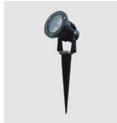
GPS-21 Dimension: 75xH280mm Lamp: LED 3W / 5W Material: Aluminum+Glass IP65
