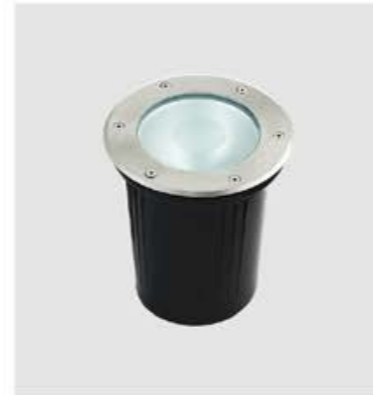
GPS-407 Dimension: 170x205mm Lamp: E27 Voltage: 220-240V Material: Aluminum+Glass+ Stainless steel+Plastic
