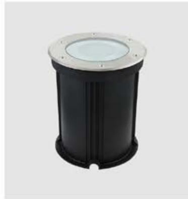
GPS-387 Dimension: 210x235mm Lamp: LED 30W Voltage: 85-265V Material: Aluminum+Glass+ Stainless steel+Plastic
