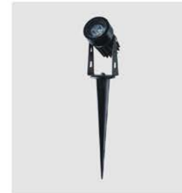
GPS-30 Dimension: 45xH250mm Lamp: LED 1W / 3W Material: Aluminum+Glass IP65
