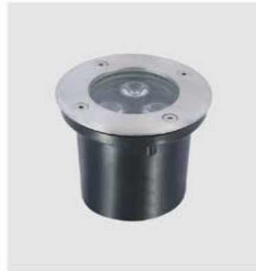
GPS-389 Dimension: 110x65mm Lamp: LED 3x1W / MR16 Voltage: 85-265V Material: Aluminum+Glass+ Stainless steel+Plastic
