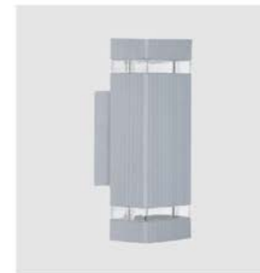
GPS-263 Dimension: 100x105x260mm Lamp: 2xE27 Voltage: 220-240V Material: Aluminum+Glass+PC
