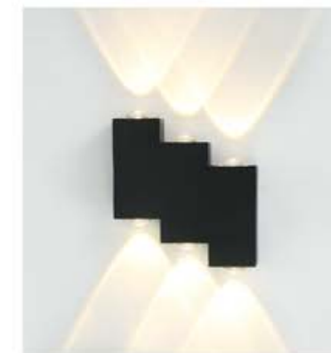
GPS-151 Dimension: 120x120x35mm Lamp: LED 6x1W Voltage: 85-265V Material: Aluminum+Lens
