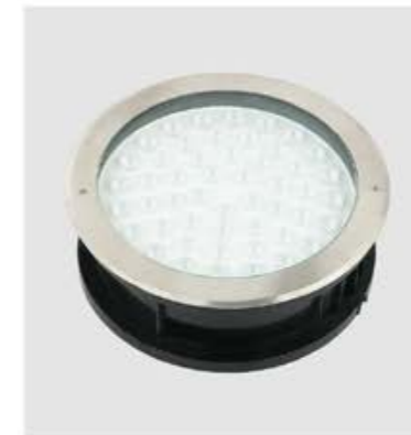
GPS-400 Dimension: 300x105mm Lamp: LED 50x1W Voltage: 85-265V Material: Aluminum+Glass+ Stainless steel+Plastic
