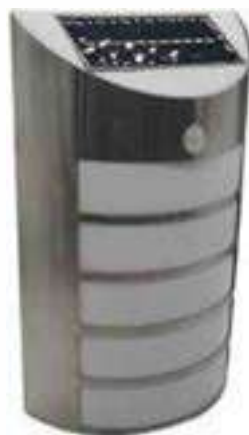
Solar Panel: Polycrystalline 5.5V 100mA 106x47mm Battery: 18650 1800mAh Light Source: 5Pcs Warm White LED Materials: PPD Dimensions: 160x75x266mm Switch : ON/OFF
