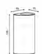
GU10 2*MAX 25W Glass Diffuser IP44 Voltage: AC 220-240V/50Hz Material:Aluminium body Size:75*95*170mm
