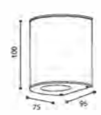
GU10 MAX 25W Glass Diffuser IP44 Voltage: AC 220-240V/50Hz Material:Aluminium body Size:75*95*100mm
