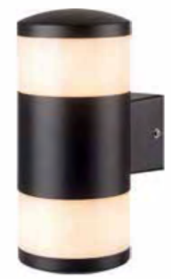
G9 2*Max 9W PC Diffuser IP44 Voltage:AC 220-240V / 50Hz Material:Aluminium Body Size: 120*89*205mm Black Grey
