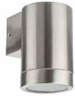
GU10 Max 35W Glass Diffuser IP44 Voltage:AC 220-240V / 50Hz Material:Stainless Steel Body
